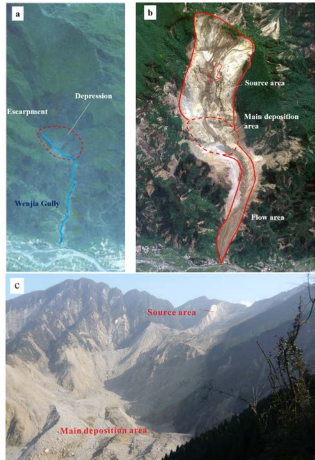
Figure 10. Sketch map of flow capacity of channel affecting on the travel distance of the Wenjia Gully channelized rock avalanche: (a) before the earthquake; (b) after the earthquake; (c) photo taken on deposition platform after the earthquake. The red arrow shows the sliding direction of source mass. The red dotted line in (a) indicates the original depression on the travel path of the rock avalanche, where debris deposition of about 30 million m^3 was stored after the earthquake (shown in b); more detailed information is shown in (c).
